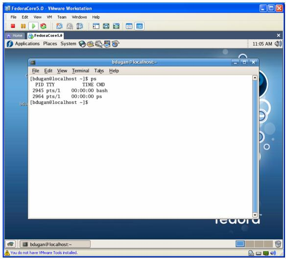
The first process is "bash", that's the name of the shell you are running inside the x-term. The second process is the "ps" command itself..
