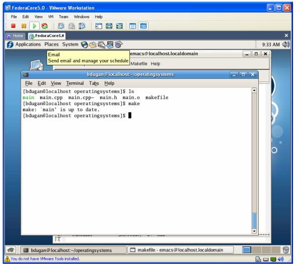
What happened? The make program determined that nothing needed to be done based on the date/times that the files used to build main were created. The timestamps for the main.cpp and main.h files were older than then main.o file. The main.o timestamp was compared against the main executable timestamp and it was found to be older. Nothing needed to be done!
