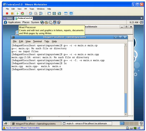
We can't run the program yet because we have an OBJECT file (main.o) not an EXECUTABLE file. To create an executable file, we need to run the linker:
