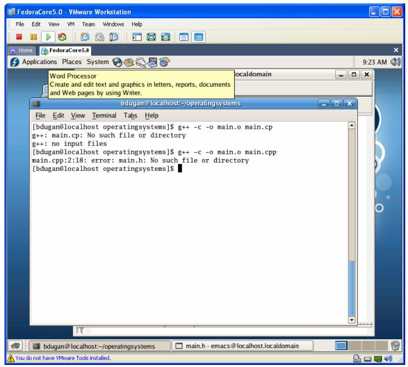
What happened? It looks like the compilation failed because the compiler couldn't find the include file "main.h". You can fix this by adding "-I." to the compiler command:
