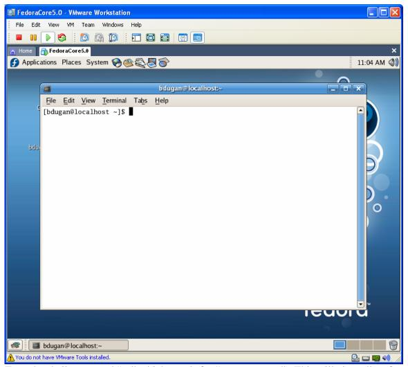
Type the shell command "ps" which stands for "process status". This will give a list of processes that are under the control of the shell you just created. You should see two of these:
