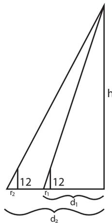
Fig. III-1-4.  $h = 12d_1/r_1 = 12d_2/r_2$ . If  $\Delta = d_2 - d_1$ , then  $h = 12\Delta / (r_2 - r_1)$ , as stated. Also,  $d_i = r_i \Delta / (r_2 - r_1)$  for  $i = 1, 2$ .
