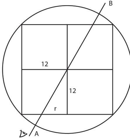
Fig. III-1-1. Diagram of astrolabe.  $AB$  represents the alidade, and  $r$ , measured on a scale of 12, is the gnomonic umbra recta.
