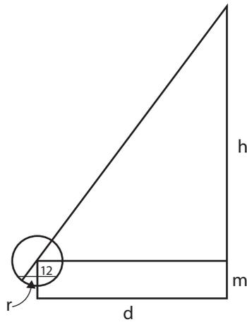
Fig. III-1-3.  $12:r = h:d$ , so  $h = 12d/r$  and the height of the hill is  $h + m$ .
