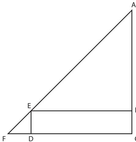
Fig. III-1-2.  $A$  is the top of the hill,  $E$  is the eye of the observer, and angle  $AEB = 45^\circ$ . Thus the height of the hill is  $AC = AB + BC = CD + ED$ . Alternatively, the astrolabe can be turned around to locate  $F$  and obtain  $AC$  as  $CD + DF$ .
